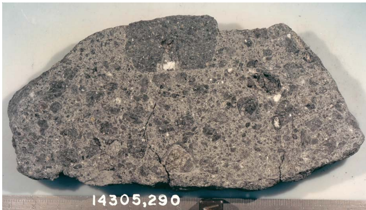
Figure 1: Sawn surface of 14305 showing dark clast in lighter matrix. Cube and scale are in cm. NASA S86-30442.
