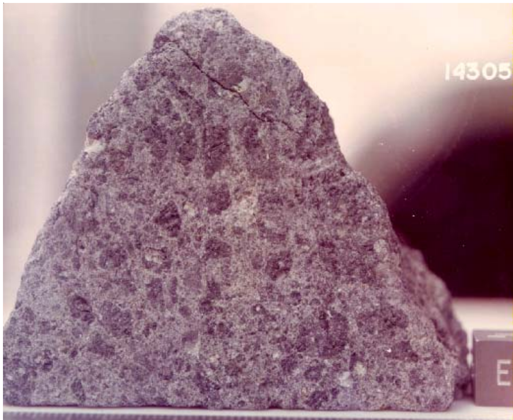
Figure 18: Sawn interior surface of 14305,30 (display piece) illustrating dark microbreccia clasts in light matrix. Cube is 1 inch. NASA photo #S77-21471.
