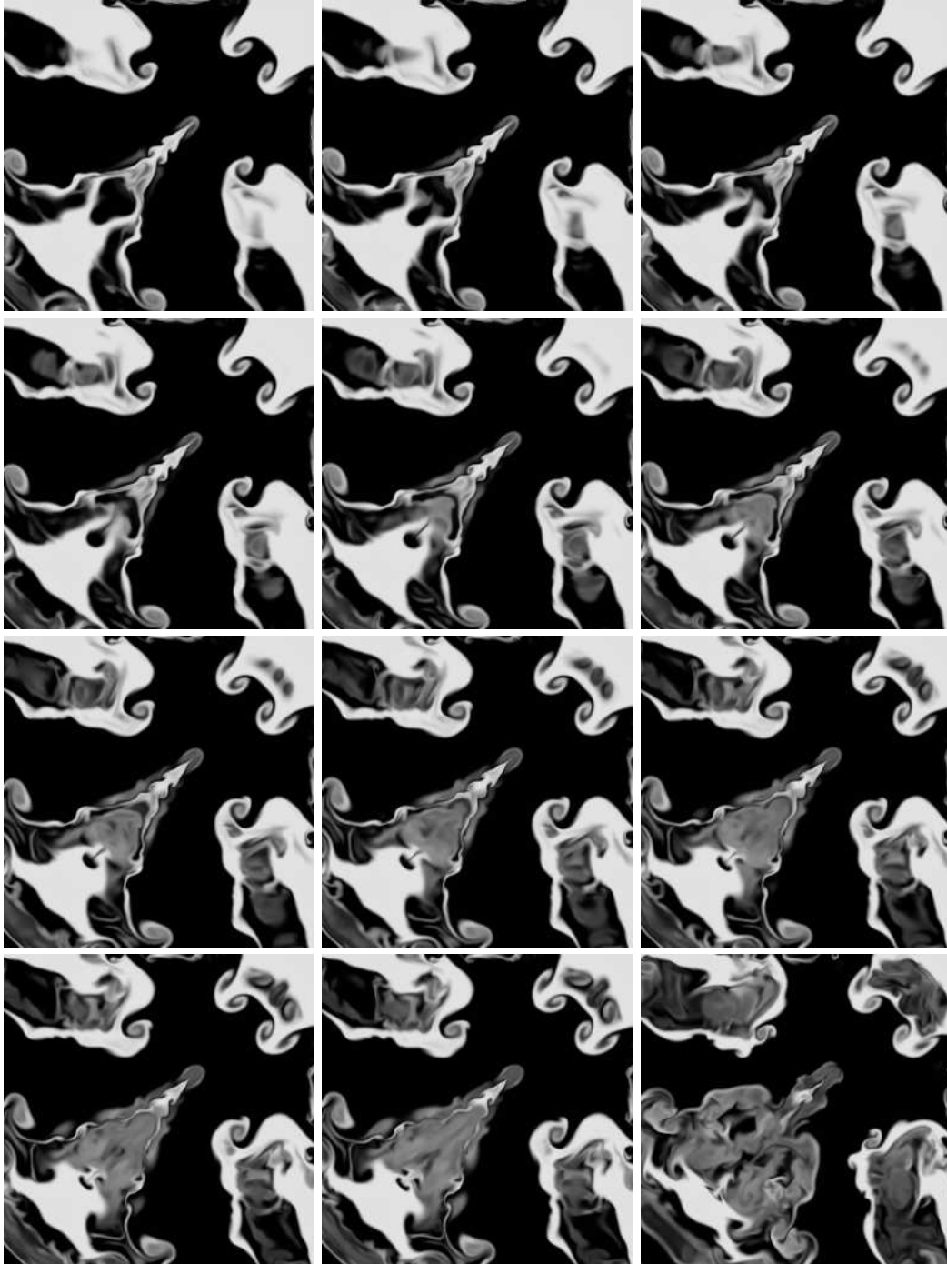
Figure 1. Example turbulence images, each of size 256 \times 256 pixels, corresponding to different time steps in the simulation. The time evolution is ordered by row. The first eleven correspond to consecutive time steps, while the last one is ten time steps after the eleventh time frame.
