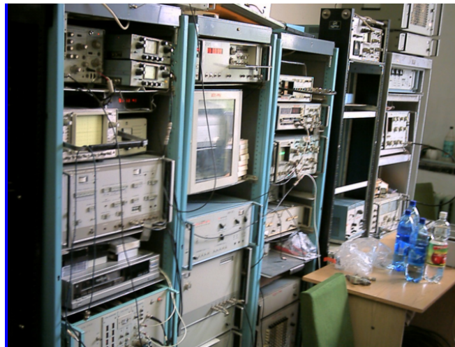
Figure 2. Recording terminals, base band converter, sampler, synthesizers, rubidium frequency standard, oscilloscopes, gauge of frequency, gauge of time intervals, spectrum analyzer, power supplies, paper recorder.
