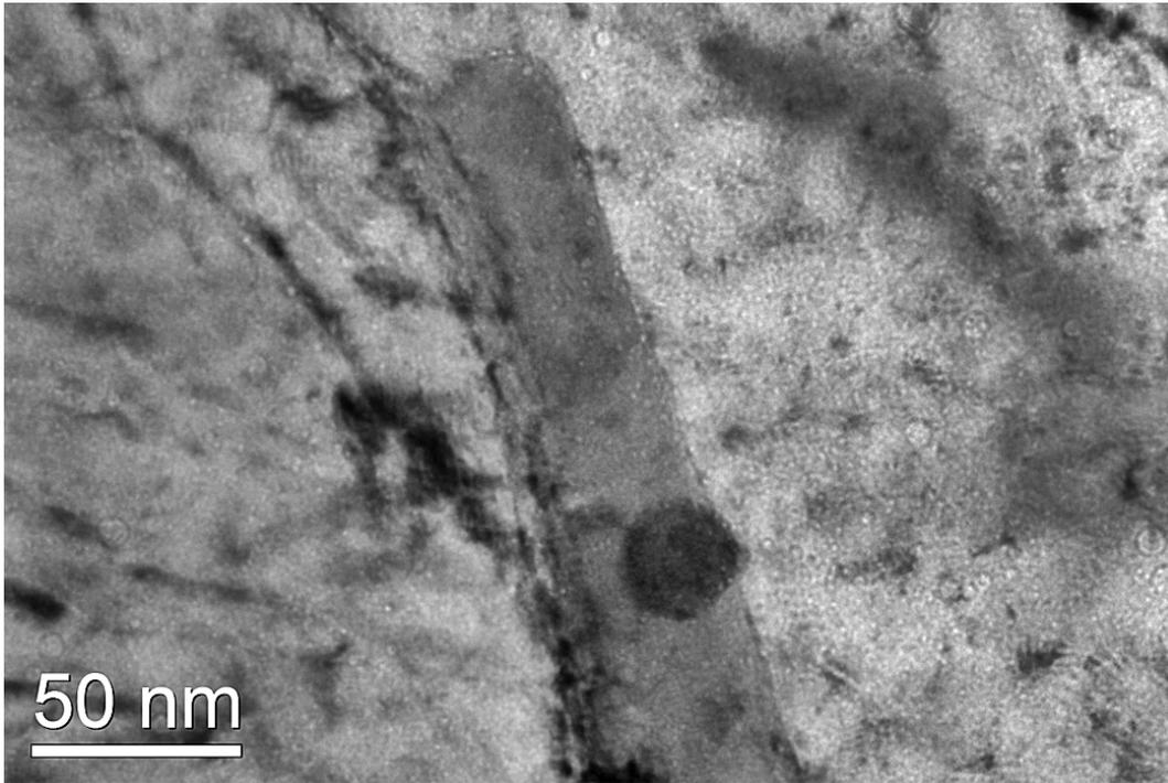
Figure 5 Cavity formation in the precipitate interface in AT F82H irradiated to 9 dpa and He-implanted to 380 appm at 500 °C.
