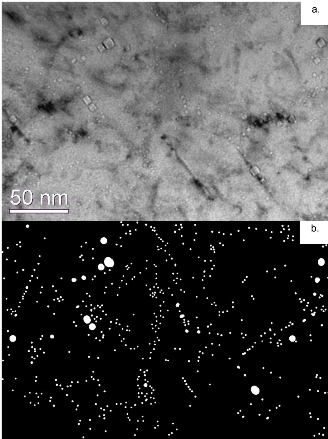
Figure 2 a) 512 nm under-focused TEM image for cavity structure in CW F82H-mod.3 irradiated to 9 dpa and He implanted to 380 appm at 500 °C, and b) a map for the features identified as bubbles by through-focus image analysis
