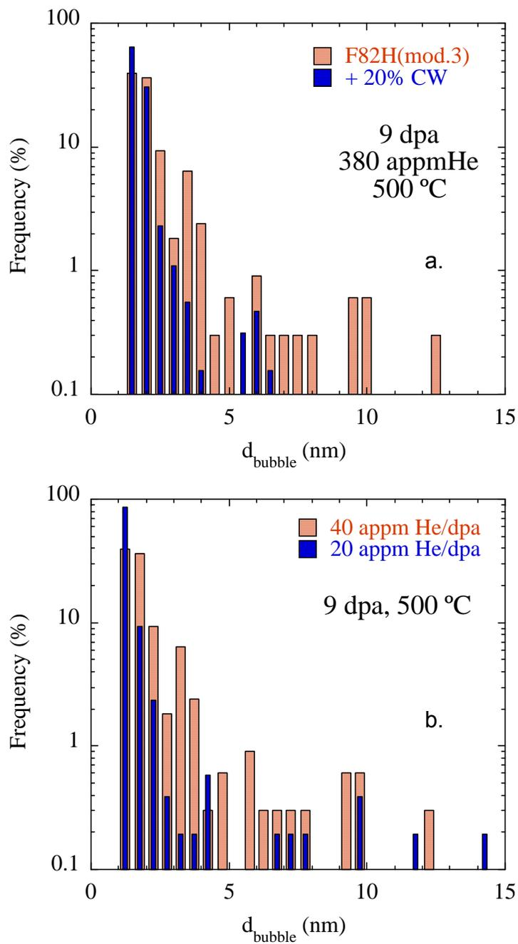
Figure 3 Cavity size distribution in a) AT and CW F82H mod.3 irradiated to 9 dpa and He-implanted to 380 appm at 500 °C, and b) at two different He/dpa ratios in AT F82H mod.3 irradiated to 9 dpa at 500 °C.
