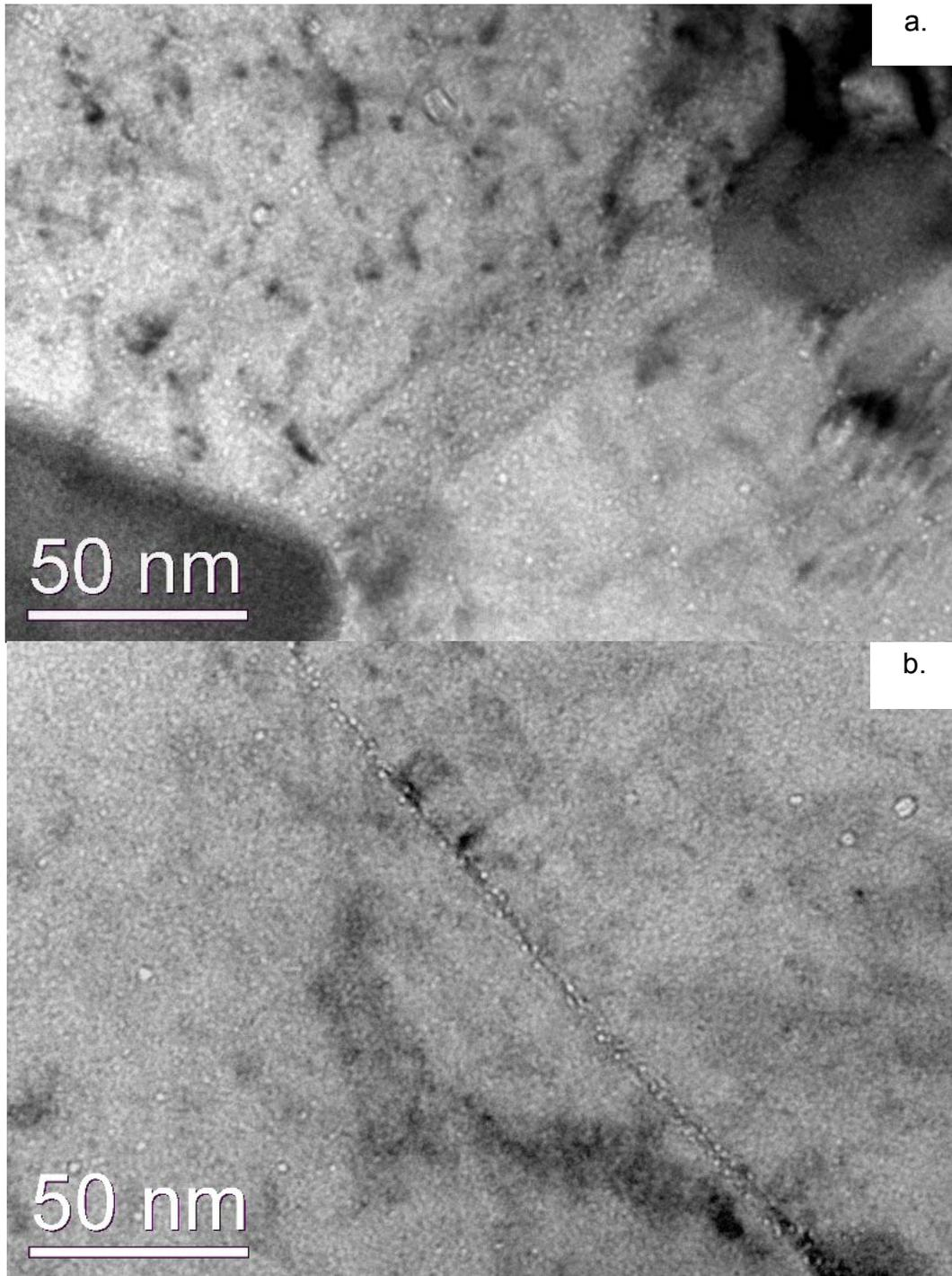
Figure 4 Cavity formation at grain boundaries in a) CW F82H mod.3 irradiated to 9 dpa and He-implanted to 380 appm at 500 °C, and b) AT F82H mod.3 irradiated to 9 dpa and He-implanted to 190 appm at 500 °C.
