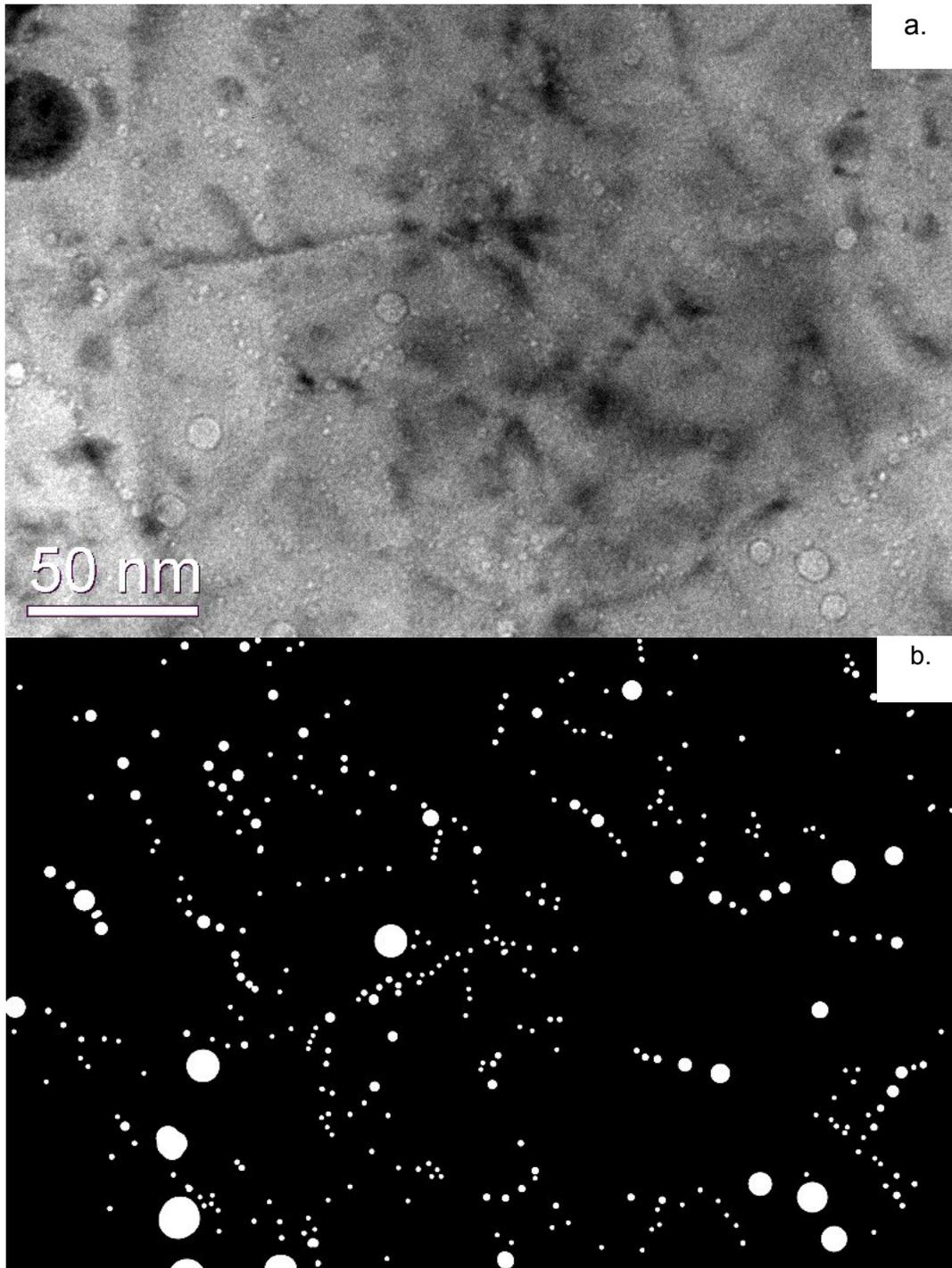
Figure 1 a) 512 nm under-focused TEM image for cavity structure in AT F82H-mod.3 irradiated to 9 dpa and He implanted to 380 appm at 500 °C, and b) a map for the features identified as bubbles by through-focus image analysis
