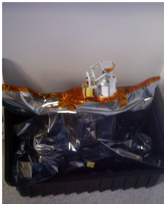
Figure 16. Mini-Corer Hydrogen Peroxide Exposure Test Set-up Detail
