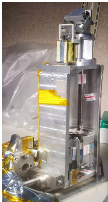
Figure 16. Mini-Corer Hydrogen Peroxide Exposure Test Set-up Detail
