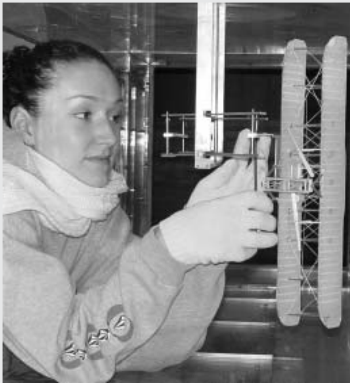
Kristi Stavros, aeronautical engineering student at Cal Poly, works on a 1903 Wright Flyer model in the 2-foot-by-2-foot slow-speed wind tunnel.
