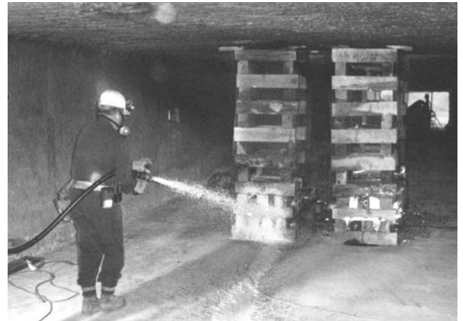
Figure 10 —Use of gas-enhanced foam during crib block Test 4.
