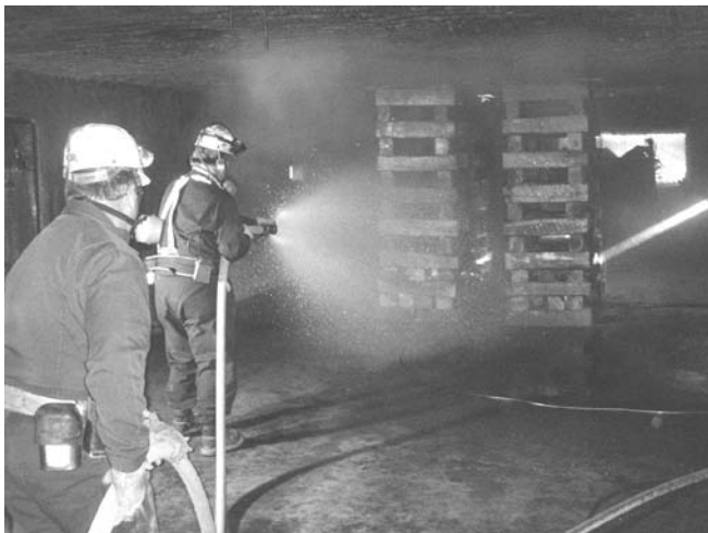
Figure 7 — Use of fire hose during crib block fire Test 3.
