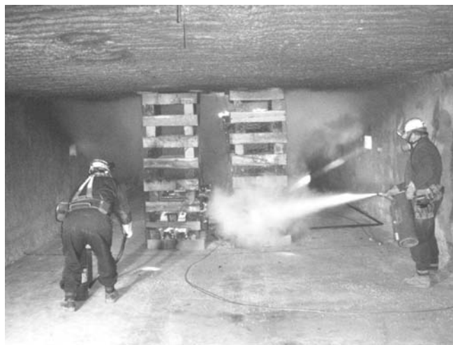
Figure 12 — Use of fire extinguishers during crib block fire Test 5.
