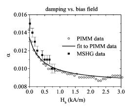
FIG. 6. Extraction of the damping parameter from PIMM data for a bias field dependent measurement and a steplike excitation pulse  $H_p$  = 320 A/m(4 Oe) (open circles). The squares show the extracted Gilbert damping parameter of the vector resolved data. The solid line shows the CBB fit to the PIMM data with a dynamically determined anisotropy of 430 A/m.
