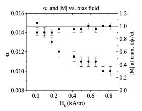
FIG. 5. Damping parameter  $\alpha$  and  $|\mathbf{M}|$  as a function of applied bias field. The filled squares show the absolute value of  $\mathbf{M}$  at the point in the time trace where the rate of magnetization change  $d\phi/dt$  is maximum. The damping parameter  $\alpha$  (filled circles) was obtained by fits of the data using the LLG model
