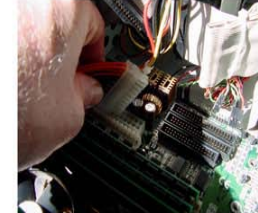
While Holding Pressure on the Locking Clip Pull Straight Upward and remove the Plug
