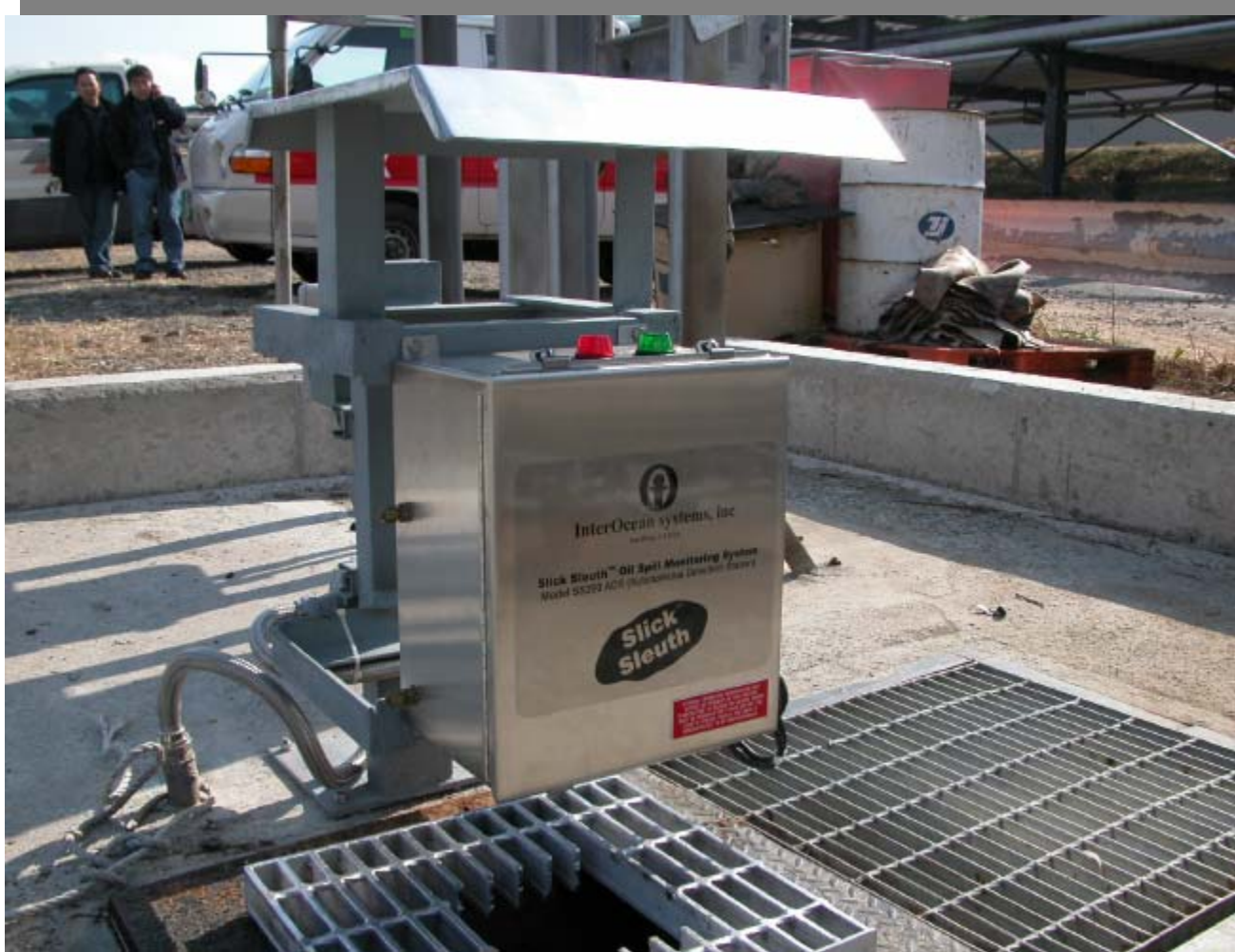
Autonomous Spill Detection Sensor ‘Peering’ Down Into Refinery’s Sewer (photo courtesy of SK Oil, S. Korea)
