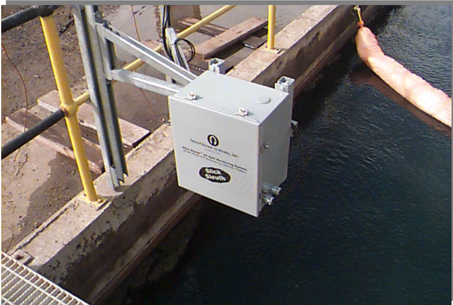
Autonomous Spill Detection Sensor Station (5 Stations Total) photo courtesy of Shell Australia
