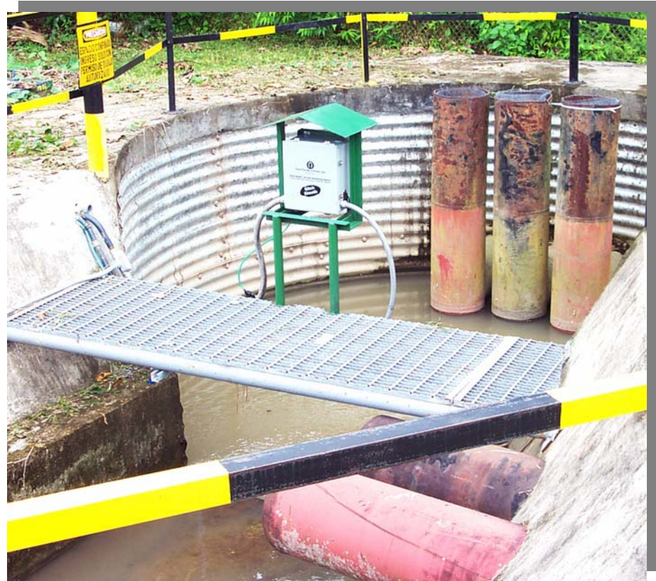
Real Time Monitoring of Outfall Points at Production Facility in South America
