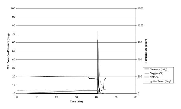
FIGURE 11. GAS AND TEMPERATURE TRACES FOR TEST 6
