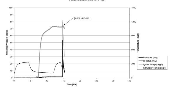
FIGURE 19. GAS AND TEMPERATURE TRACES FOR TEST 17
