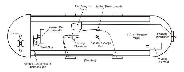
FIGURE 1. PLAN VIEW OF PRESSURE VESSEL SETUP
