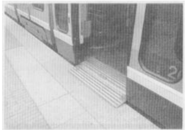
Figure 32. Grenoble/Rouen/Paris GEC-Alsthom LF-LRV powered ramp (photo).
