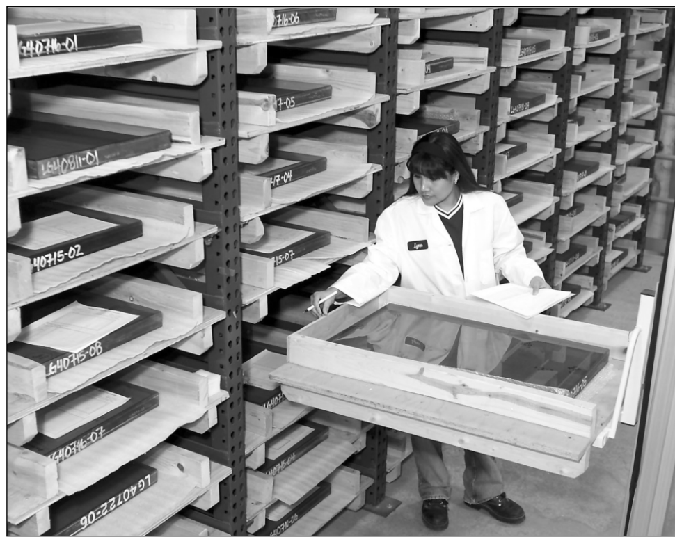
Lynn Yankiling, a quality assurance inspector at Hoya, examines the most recent batch of laser glass. The glass slabs will be used in the National Ignition Facility.
