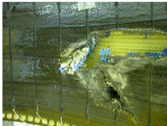
Figure 23. Series of pictures depicting 1) engine half case as received, 2) application of masking tape used to define sensor grid, 3) first set of finished grid lines, 4) completed case with sensor grid ready for impact test, 5) case after first impact event, 6) case after second impact event.
