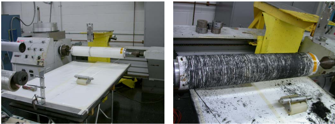
Figure 22. Filament winding set-up for producing a conductive glass tow using a conductive carbon nanofiber coating.
