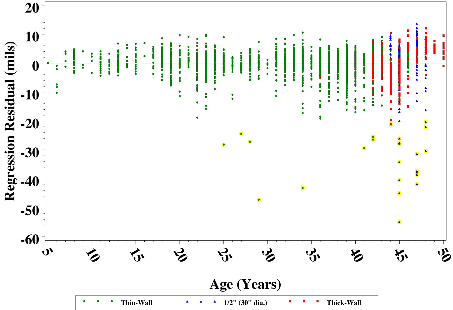
Figure 35. Residuals from minimum thickness regression. Residuals below -20 mils are highlighted (yellow) and corresponding cylinders are not used to compute Table 14B.
