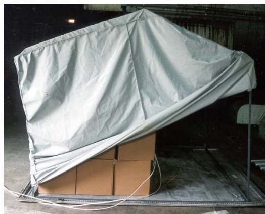
The FAA has conducted extensive tests of fire-resistant cargo covers. This photo shows a partially loaded pallet before the test cover was fully lowered.
