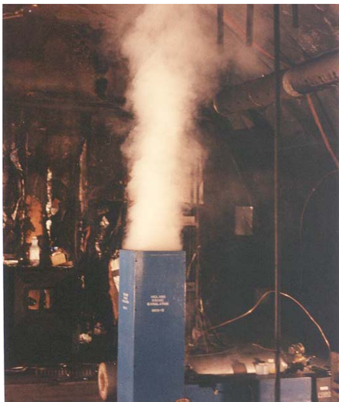
When testing fire suppression systems for cargo compartments, the FAA uses a combination of helium and theatrical smoke to produce a plume with buoyancy properties similar to the plume from a small fire. Generating smoke for as little as fifteen seconds with this smoke generator caused smoke detectors to alarm in less than one minute for all the locations tested.
