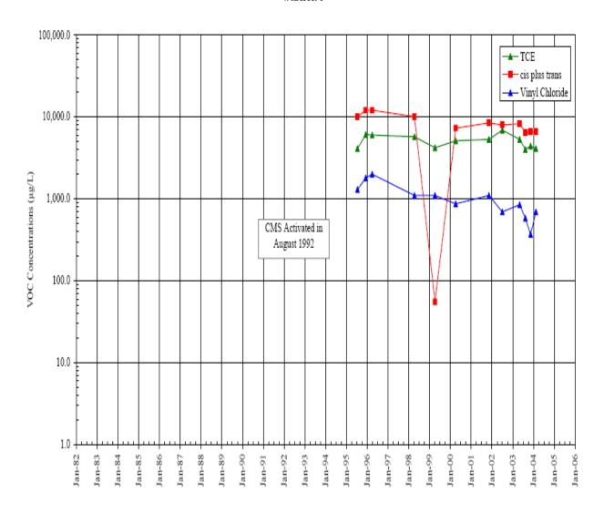
Figure 6. Presence of VOC concentrations ( $\mu g/L$ ) in recovery well HYR-1 from 1995 to 2004 at BSB property, Kent, Washington (source BSB Diversified draft remedial investigation (RI) report).<sup>1</sup>
