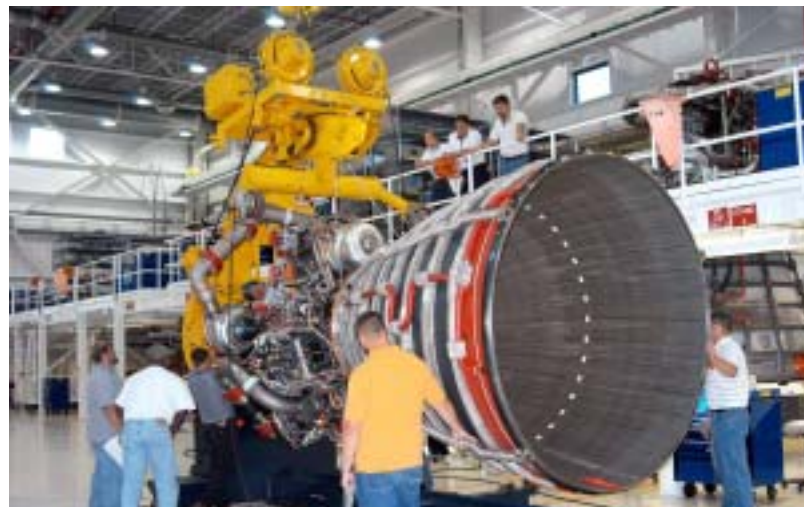
IN THE Space Shuttle Main Engine (SSME) Processing Facility, Boeing-Rocketdyne employees secure SSME 2058, the first SSME fully assembled at KSC, onto an engine stand. Each engine is 14 feet long, with a 7.5-foot-diameter nozzle.
