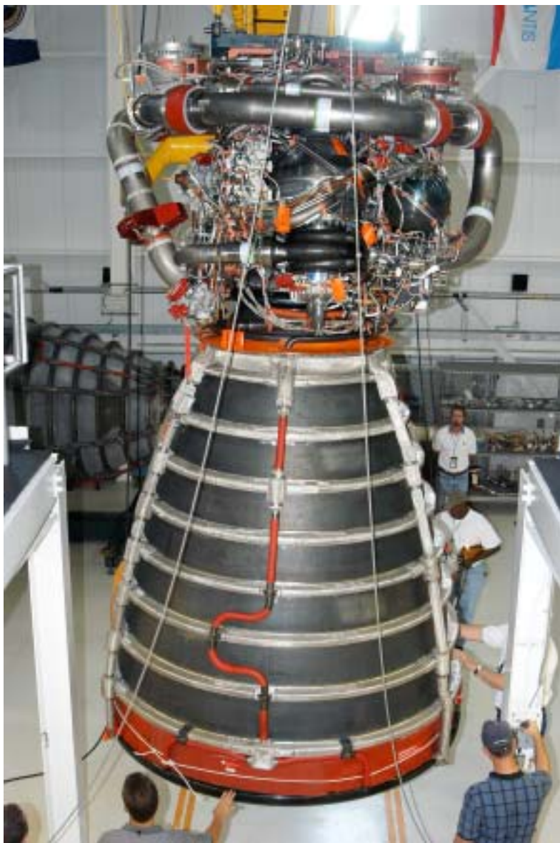
IN THE Space Shuttle Main Engine (SSME) Processing Facility, Boeing-Rocketdyne employees secure SSME 2058, the first SSME fully assembled at KSC, onto an engine stand. Each engine is 14 feet long, with a 7.5-foot-diameter nozzle.
