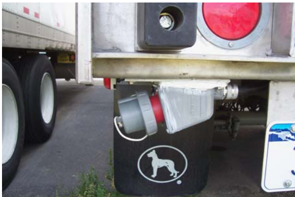
Figure 5-6. Side View of New Trailer Plug Assembly
