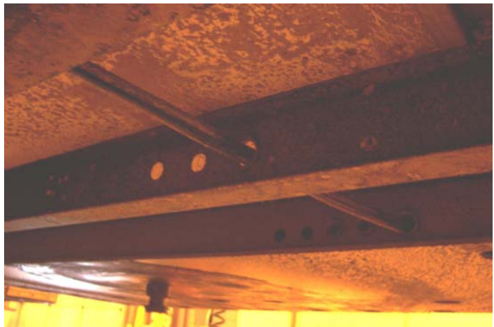
Figure B-1: View of upper coupler assembly with holes for fuel line and power cable pass through
