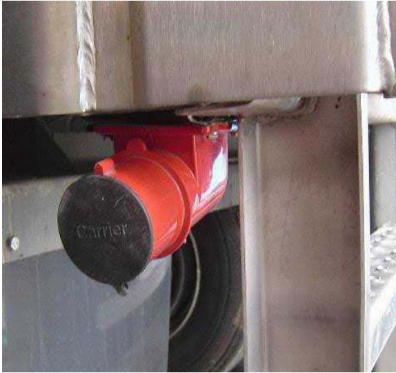
Figure 5-2: Original Trailer Plug Connection – Front View
