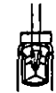
C. Put the igniter all the way into the engine. Do not bend. Igniter must touch propellant.
