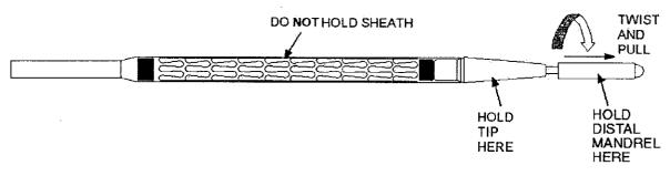
(Hold the tip to remove the distal mandrel.)
