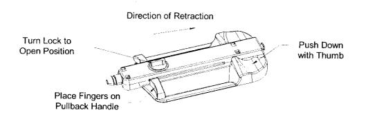
With the guide position fixed, deploy with one hand. PUSH DOWN on the thumb groove and retract the pullback handle.
