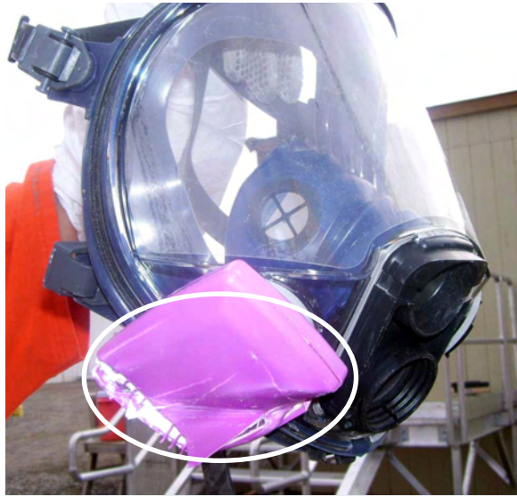
Figure 1-2. Damage to pink filter on painter's respirator
