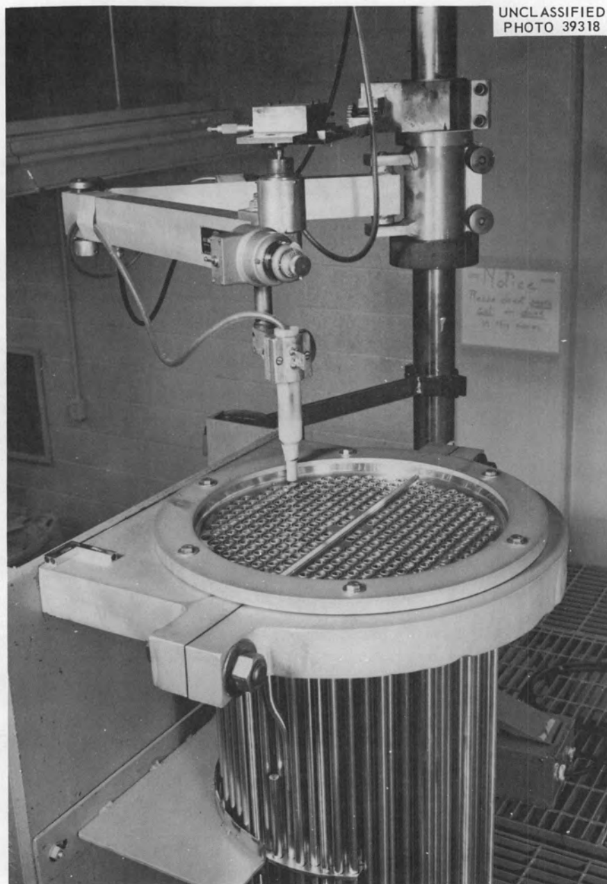
Fig. 11. Specially Built Torch Positioned for Welding.
