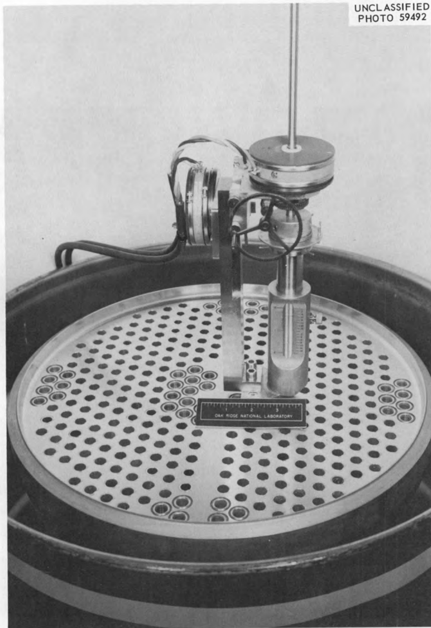
Fig. 17. Ultrasonic Probe Device Set up on Sample Heat Exchanger To Inspect Tube-To-Tube Sheet-Brazed Joints.
