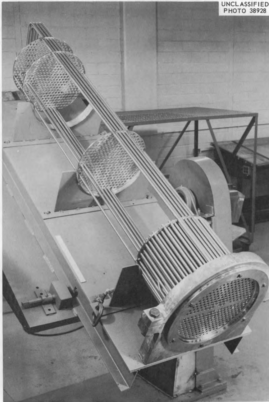
Fig. 8. Completed Sample Heat Exchanger Positioned in Welding- Inspection Fixture.
