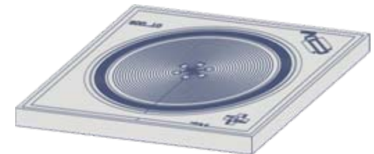
SDD 10 mm 2 chip 6 x 6 x 0.45 mm 3
