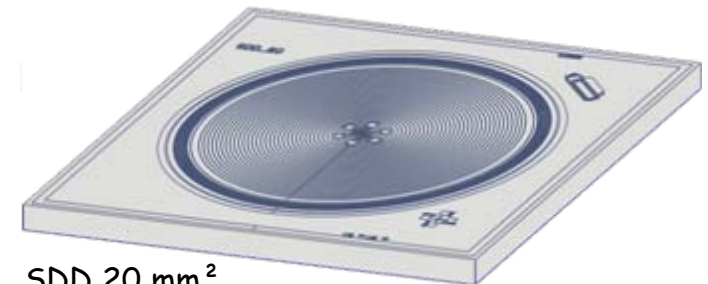
SDD 20 mm 2 chip 8 x 8 x 0.45 mm 3
