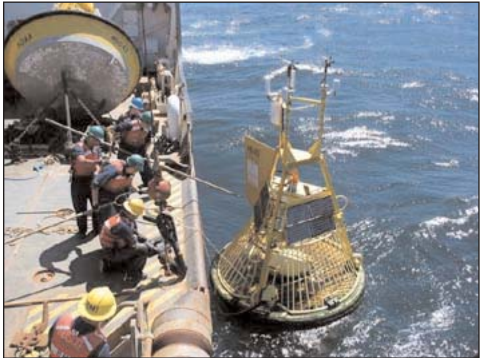
Operation in action: replacing 3-meter buoy off the coast of California.
