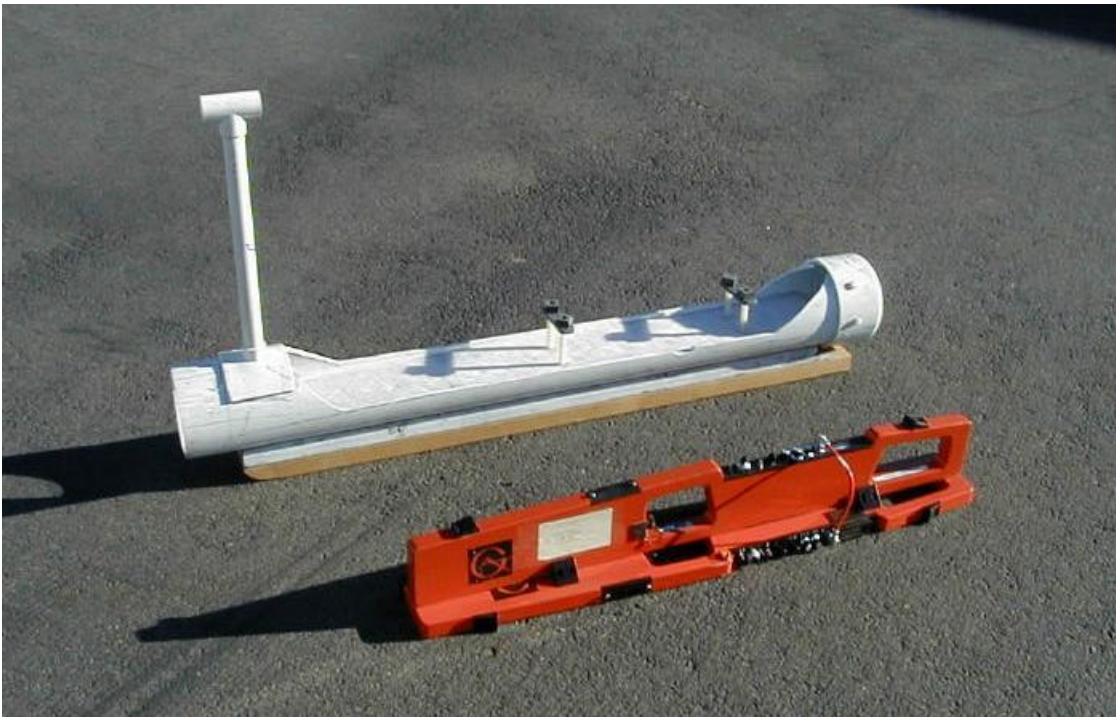
Figure 12. Finished sled with EM-38DD placed alongside the sled unit.
