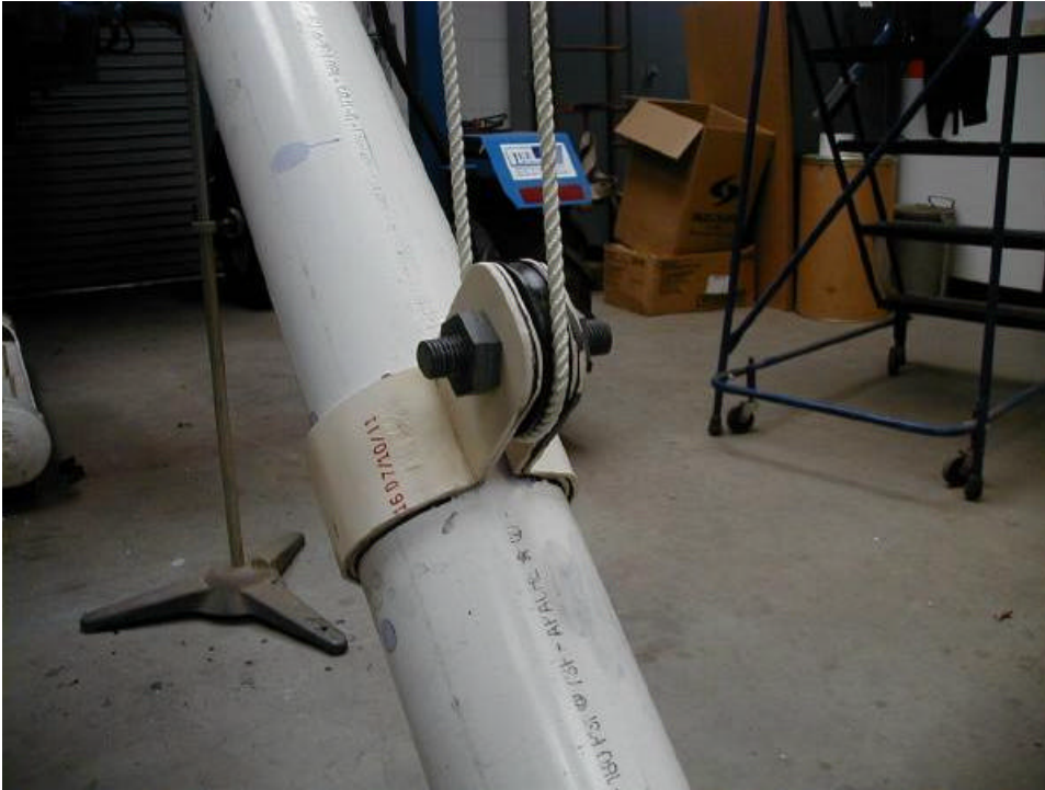
Figure 3. Close-up image of the PVC pulley used on the dog-tail extension piece.
