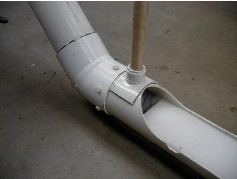
Figure 4. Close-up image of how the sled attaches to the dog-tail (using 5 PVC bolts).
