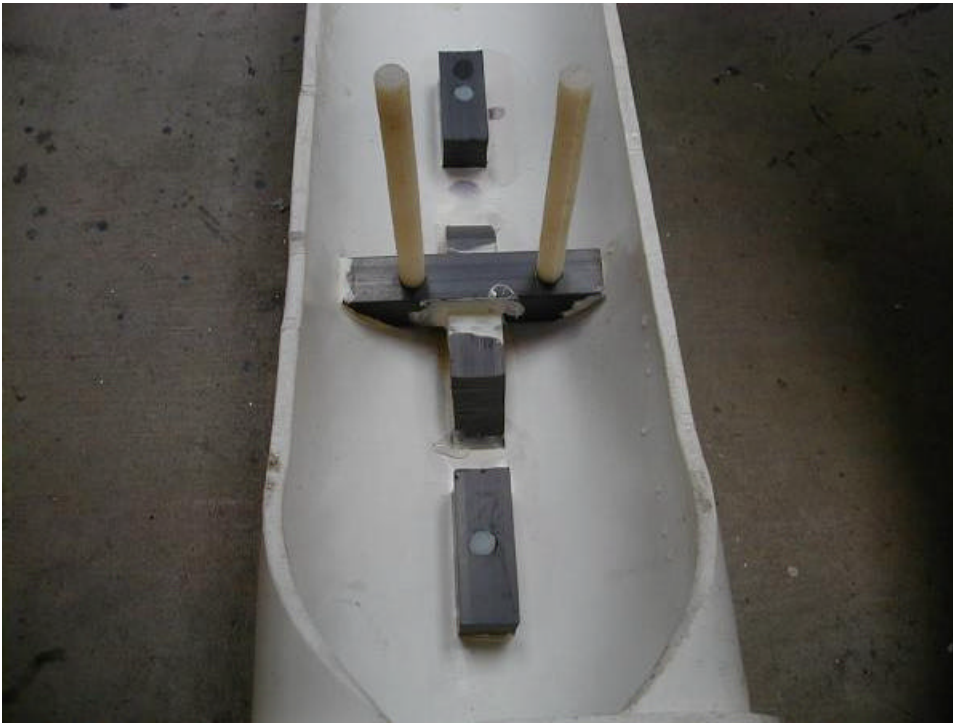
Figure 11. Close-up view of one set of EM-38DD attachment rods.
