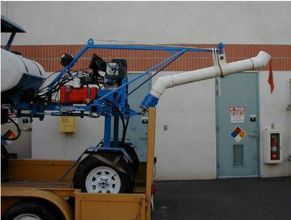
Figure 14. Hoisted, secured dog-tail extension; ready for travel.
