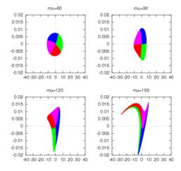
Figure 5 :  $(\delta\phi^{\circ}, \delta p/p)$  portraits after two cells for a geometrical emittance  $57\pi$ .mm.mrad, and the phase advance values :  $\mu = 60^{\circ}, 90^{\circ}, 120^{\circ}$  and 155.
