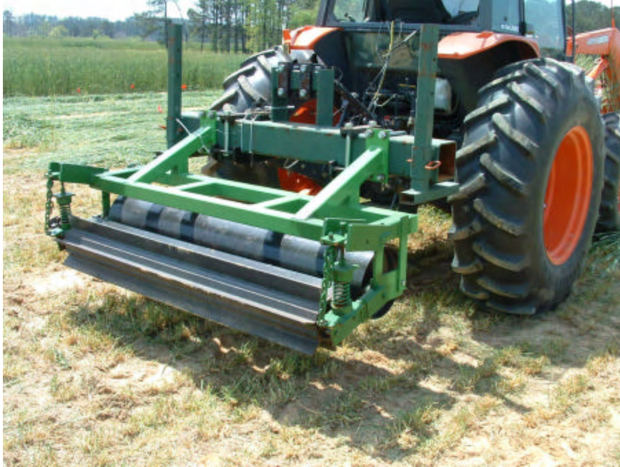
Figure 4. Two-stage roller comprised of a smooth drum and spring loaded crimping bar drum.
