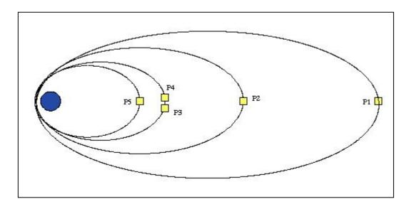
The THEMIS program has launched five satellites that will orbit earth at different distances to study Earth's magnetic field. The goal is to have them line up a few times each year so that they can study how magnetic storms are triggered and evolve in time.
