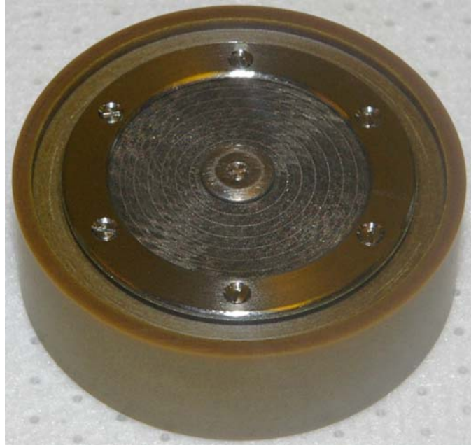
Figure 12.—Assembled oscillating-flow rig regenerator (stack of 42 disks).
