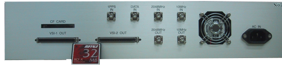
Figure 2. Rear view of ADS-3000. FPGA logic is easily programmable with a CompactFlash card, or an Ethernet port which will be equipped after the next upgrade. 2048-MHz PLL-output port and 2048-MHz input port are directly connected in most cases. 2048-MHz reference signal can be distributed to other units by using these ports.
