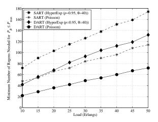
Fig. 9. Number of regenerators required to achieve a new connection blocking probability of 0.001 using DART and SART architectures with Poisson and hyper-exponential connection arrival processes.
