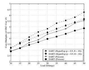
Fig. 12. Cost of DART and SART architectures as a multiple of OXC cost  ${\cal O}$  when f=0.04, for hyper-exponential and Poisson arrival processes.
