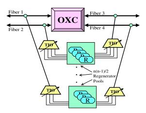
Fig. 1. Switch architecture associated with dynamically allocated regenerators and TR modules (SART architecture).
