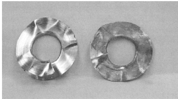
Figure 6. Coated aluminum fin (left) and non-coated aluminum fin (right) after one month test in salt-spray chamber at 35°C.
