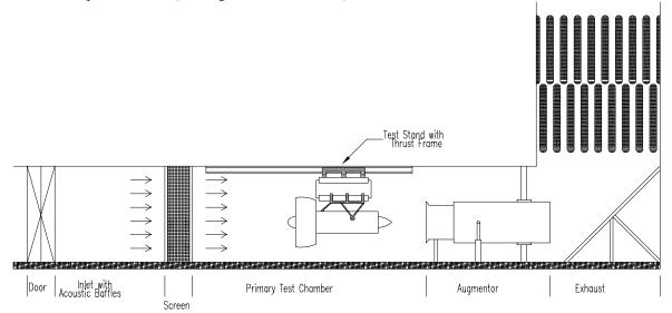
FIGURE 2-1. TEST CELL CONFIGURATION: "L" TYPE
