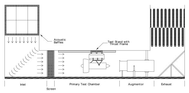
FIGURE 2-2. TEST CELL CONFIGURATION: "U" TYPE
