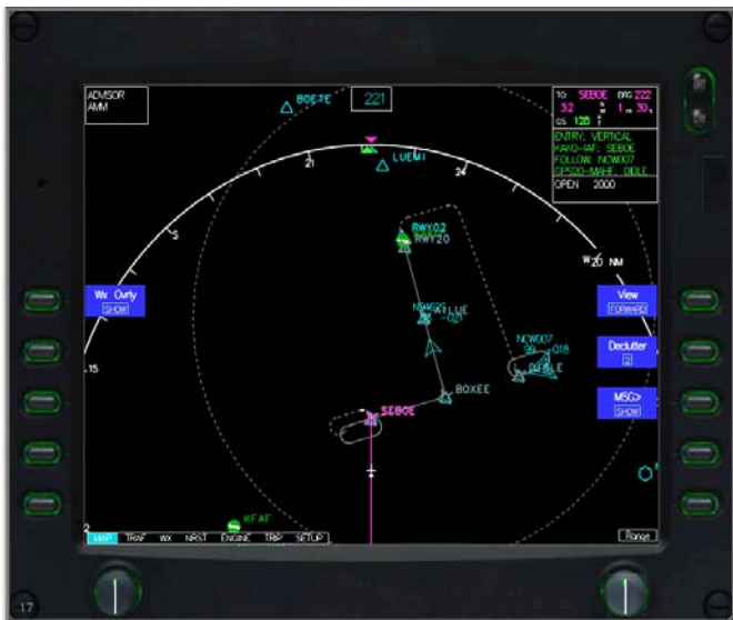
Figure 12. HVO-2 MFD (white own-ship, traffic to follow double-cyan chevron, green “Entry” message, solid line instrument approach, dotted line missed approach)
