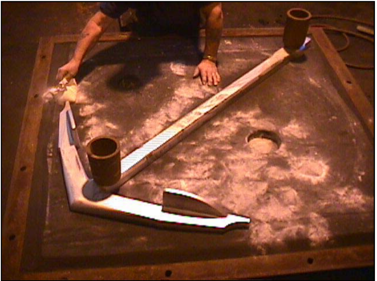
National Park Service Woodcrafter John Pydynkowski made the full-size reproduction anchor pattern in this photo. The castings were poured at the Henry Perkins Foundry of Bridgewater, MA
