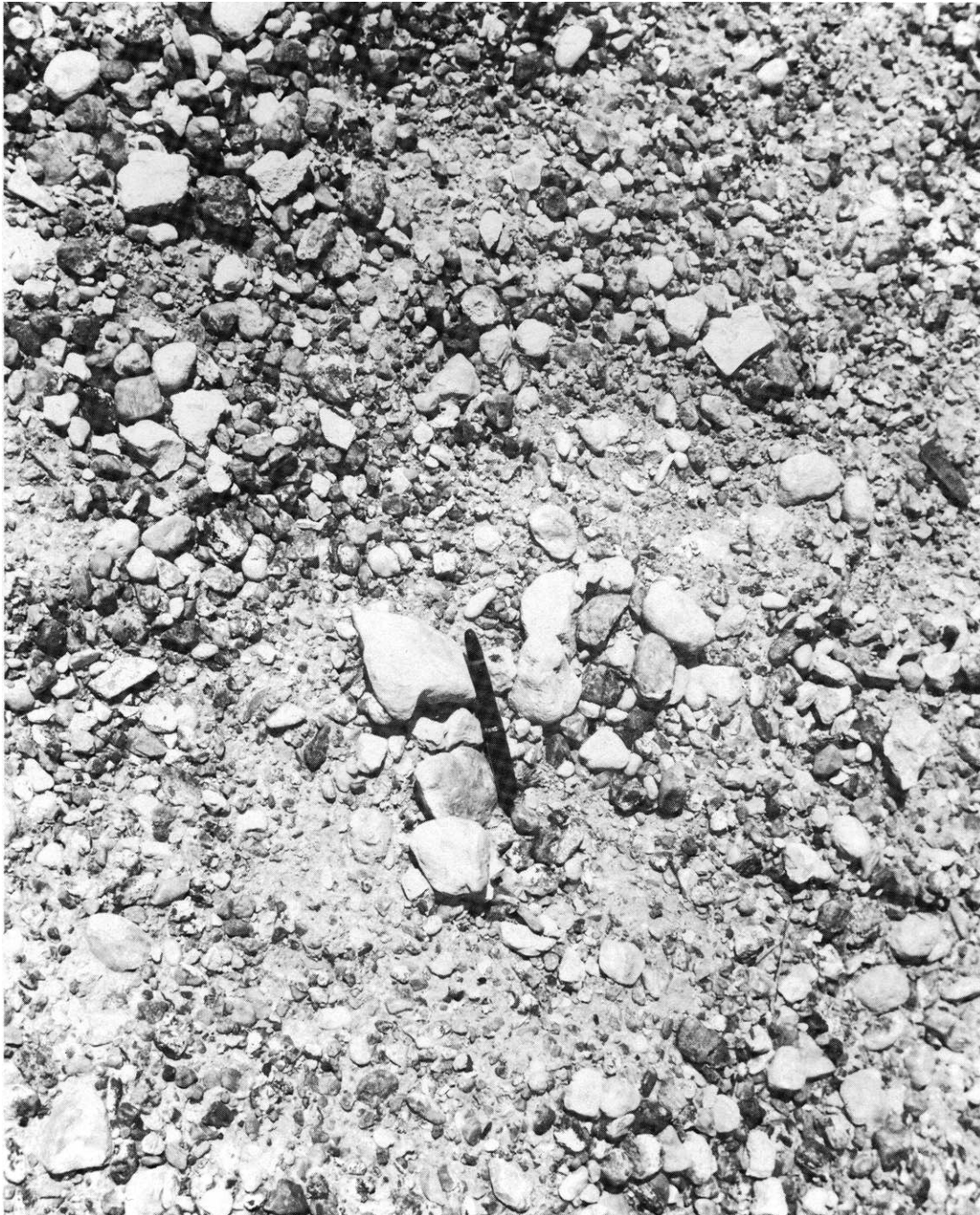
Figure 18. Closeup of Thin Elk gravel shown in Figure 17. Pen (5 1/4 inches long) indicates size of largest cobbles.
