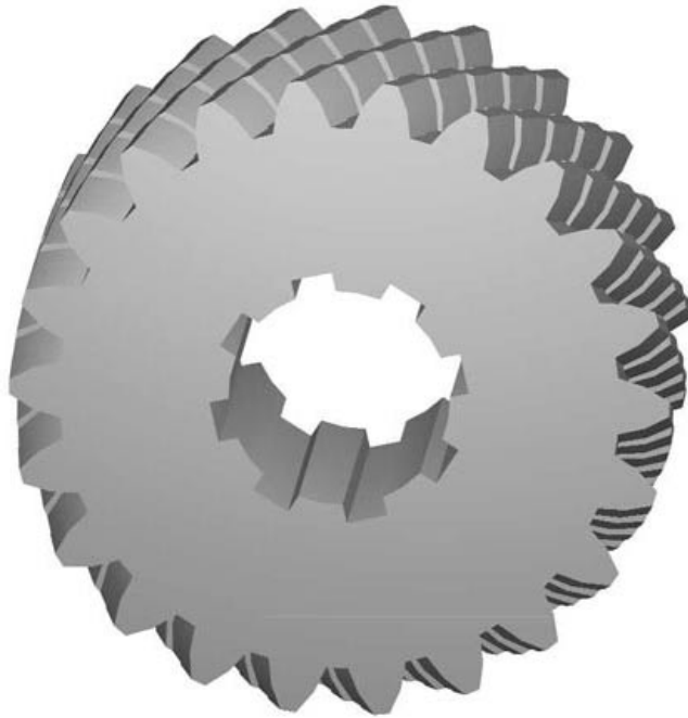
Figure 1.—Illustration of a shaver as a helical gear with gashed teeth.
