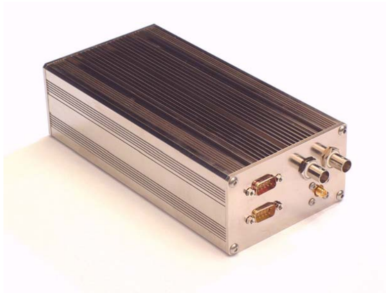
Figure 3.1.5 : WLAN Base-station unit
