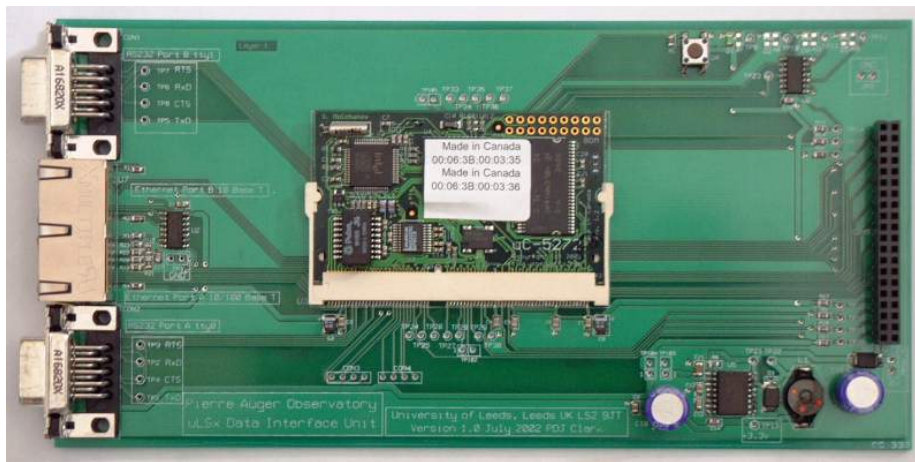
Figure 3.1.7 : Micro-LSX unit provides E1 to TCP/IP conversion
