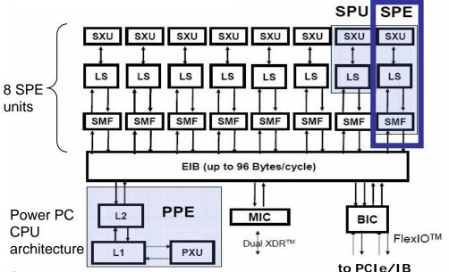
Each of the 8 SPEs are 128 bit (e.g. 2-way DP-FP) vector engines w/ 256KB of Local Store (LS) memory & a DMA engine.
