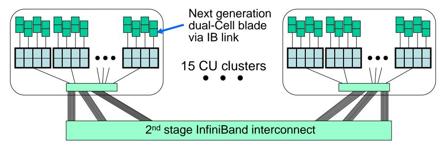
Cell blades are attached via direct IB links to 138 nodes of each CU
