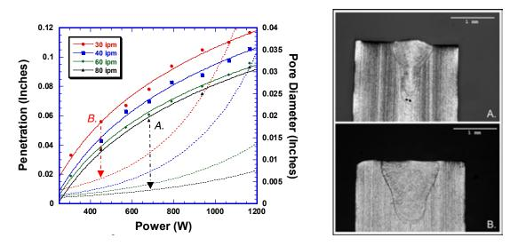
Figure 3: Argon shielded sharp focus Rofin CW LBW's with 120 mm lens. 250 - 1200 W, 30 - 80 ipm (Left). Transverse micrographs (right) at 80 ipm 680 W (A) and 30 ipm 450 W (B) having equal penetration of 0.058".
