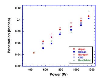
Figure 7: Sharp focus Rofin CW LBW's at 350 – 1200 W, 40 ipm. 70 CFH flow rate.
