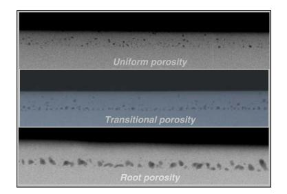
*Figure 2: X-ray Radiography identifying pore formation types for argon shielded sharp focus CW LBW's.*
