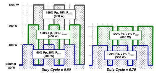
Figure 11: Schematic of SQW modulation operator defined parameters.
