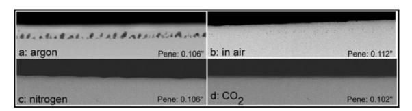
*Figure 9: X-ray radiography contrasting approximately equal penetration welds made under various gas shielding conditions. Rofin CW, 1165 W, 40 ipm. 70 CFH flow rate.*
