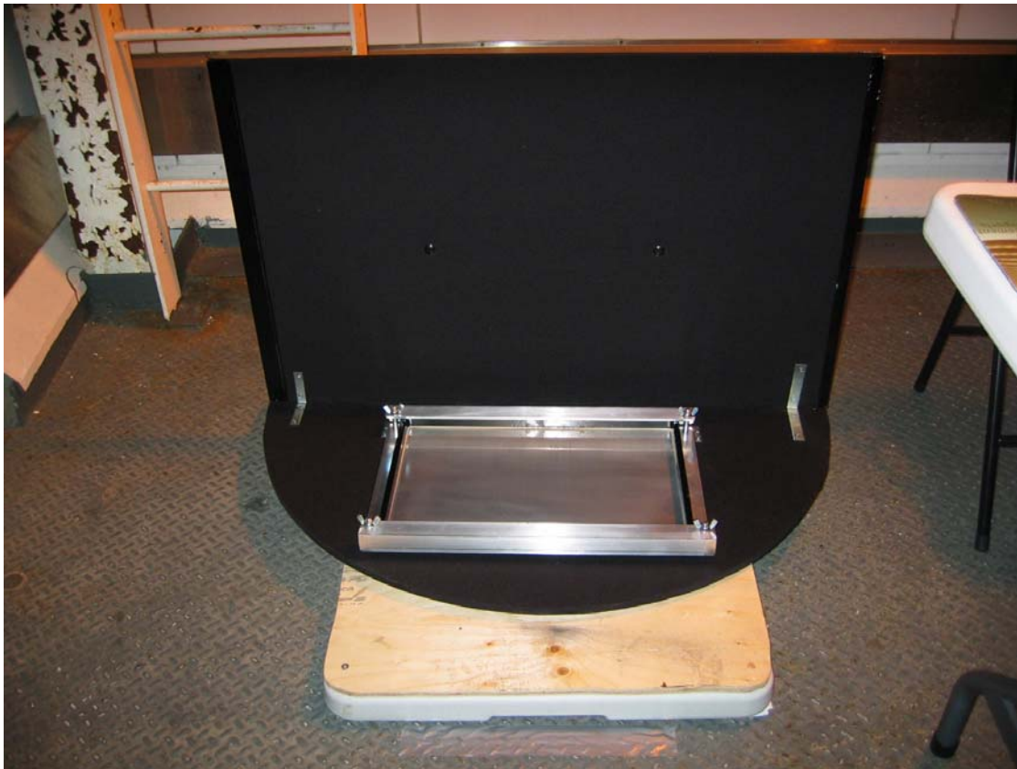
Figure 4. This image shows an unpainted aluminum panel with ice. Ice is formed on the panel and then covered with deicing fluid. The black frame and aluminum clamps hold the deicing fluid in place.
