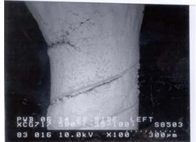
Figure 11 Optical photomicrographs of CCGA 717 I/O assembly (left) at 200 thermal cycles and their SEM Photomicrographs at 500 cycles. Some signs of damage at 500 cycles is apparent.
