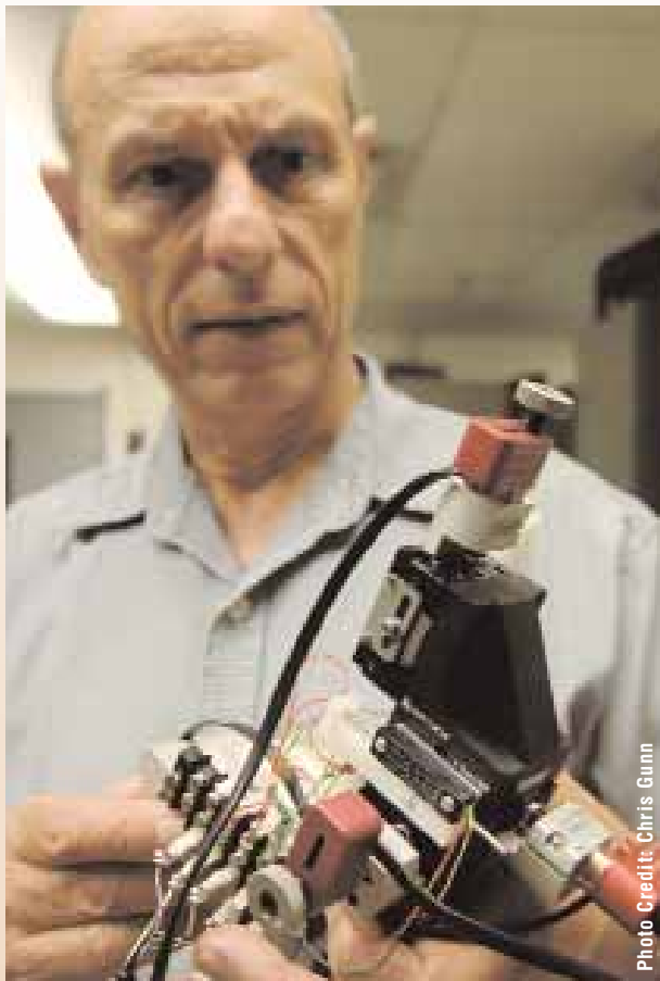
Goddard scientist Sam Floyd holds a device he used to test his concept for a Neutron/Gamma ray Geologic Tomography (NUGGET) instrument, a concept instrument that may help astrobiologists search for evidence of life on Mars.
