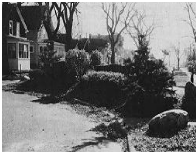
Figure 14: Permanent diagonal diverters. Source: Appleyard (1981).
