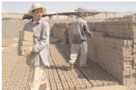
Afghan workmen make bricks at a Kabul building project rising amid the rubble left by war.
