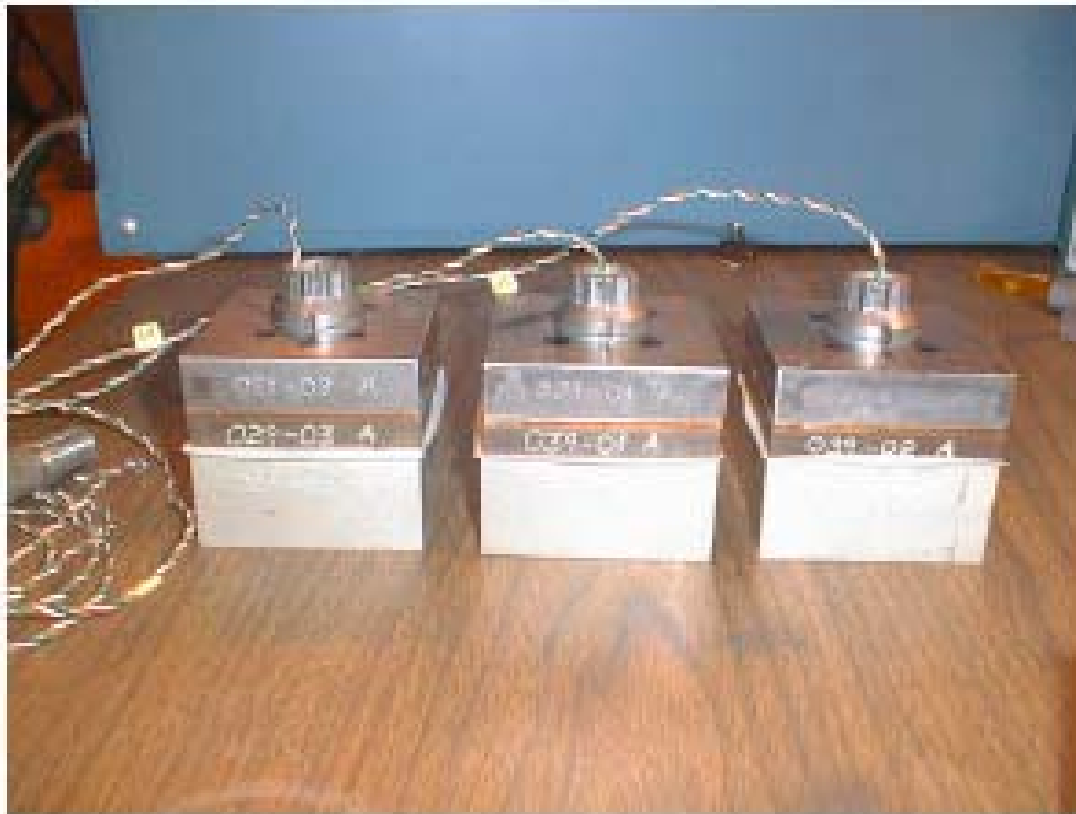
Figure 4.2-1. Example Component Test Specimens [ref. Wingate, ET Bipod Fitting Bolted Joint Attachment Design and Locking Insert Performance presentation, June 13, 2006]
