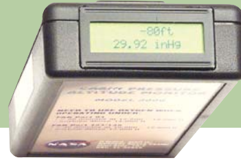
This close-up shows the pager-sized Personal Cabin Pressure Altitude Monitor developed by Jan Zysko, chief of the KSC Spaceport Engineering and Technology directorate's data and electronic systems branch.
