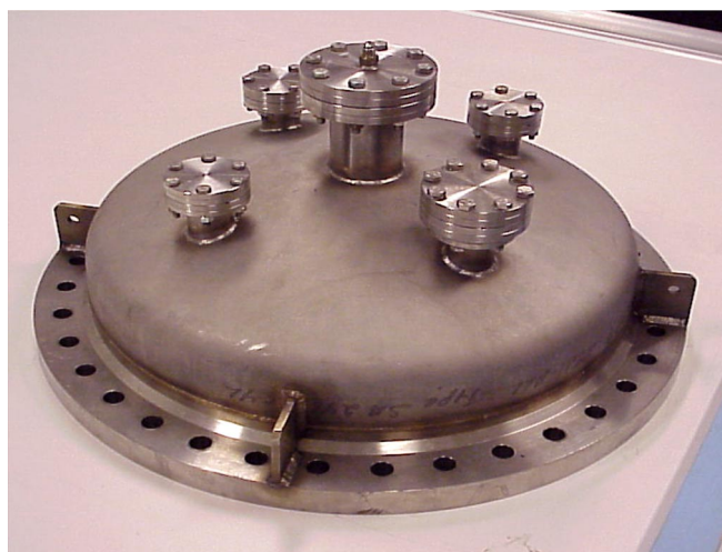
Figure A-2.—Tank lid section. (The five ports are capped off.)
