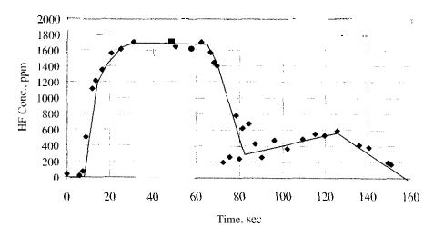
Figure 5. Sodium hicarbonate (<  $7 \mu m$ ) results (NMERI Puffer apparatus).
