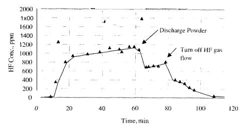
Figure 4. Sodium bicarbonate (43 to 53 µm) results (NMERI Puffer apparatusj.
