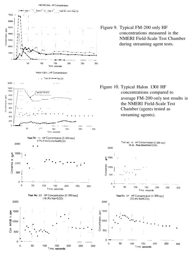
Figure 11. HF concentration versus time for selected FM-200 and sodium bicarbonate tests.
