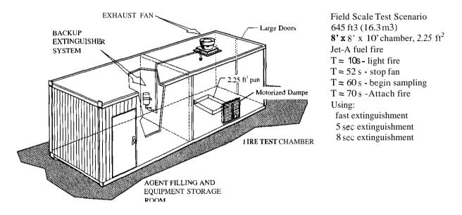
Figure 8. NMERI Field-Scale Test Chamber.
