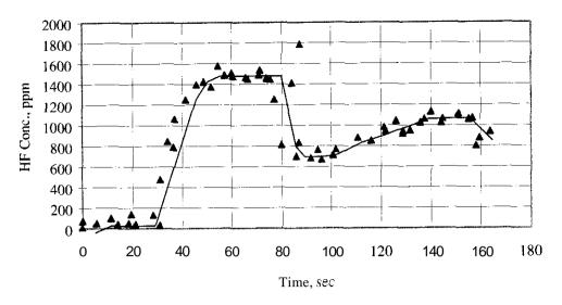
Figure 7. Potassium bicarbonate (43 to  $53 \,\mu\text{m}$ ) results (NMERI Puffer apparatus).
